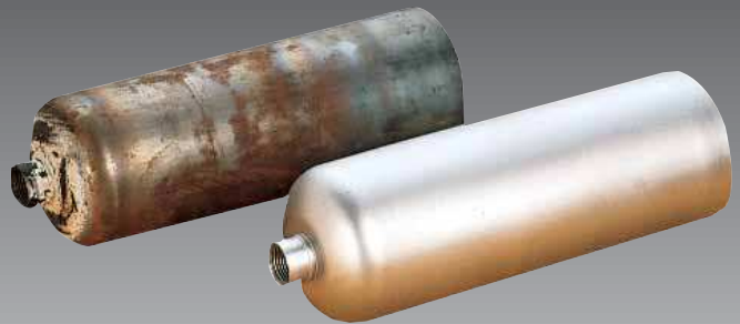
Cylinder surface profiled with aluminum oxide
